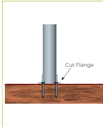
**For Millwork Counter Concealed Fastener (not for cantilever units)**
